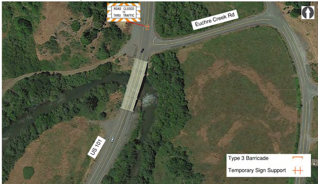
Euchre Creek Road (MP 316.9) – Northbound traffic
